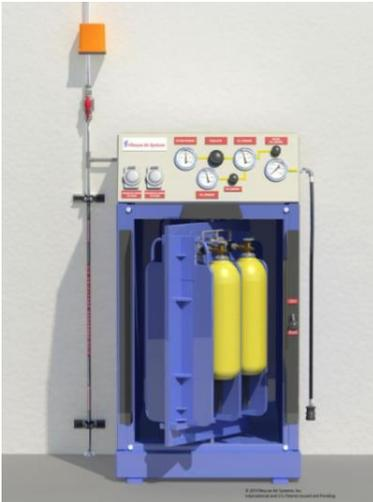
FARS is a permanently installed arrangement of piping, valves, fittings, and equipment to facilitate the replenishment of breathing air in self-contained breathing apparatus (SCBA) for firefighters engaged in emergency operations. The code change recommends that local ordinances should adopt the implementation of the firefighter air replenishment systems based on building characteristics or special hazards.
